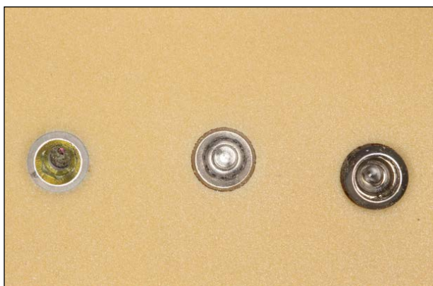
Fig 1 6-mm implants with different macrogeometries placed in the artificial bone block with type I bone quality.
