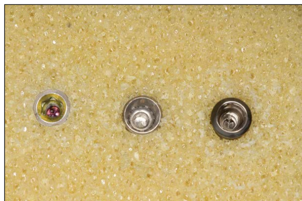
Fig 2 6-mm implants with different macrogeometries placed in the artificial bone block with type IV bone quality.
